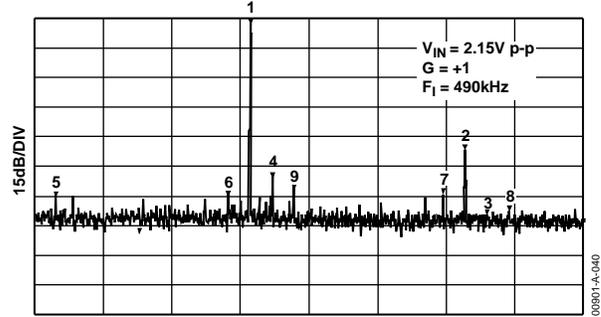
Figure 41. FFT of AD1672 Output Driven by AD823
