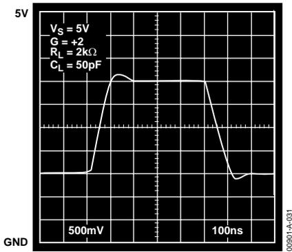
Figure 31. Pulse Response,  $V_S = 5\text{ V}$ ,  $G = +2$
