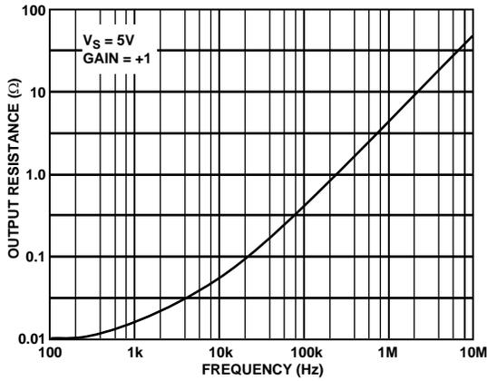
Figure 18. Output Resistance vs. Frequency,  $V_S = 5V$ , Gain = +1
