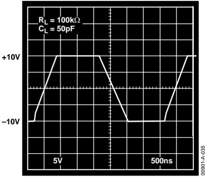
Figure 35. Pulse Response,  $V_s = \pm 15V$ ,  $G = +1$
