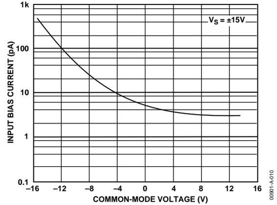
Figure 10. Input Bias Current vs. Common-Mode Voltage
