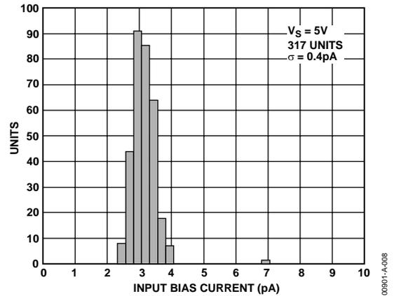
Figure 8. Typical Distribution of Input Bias Current
