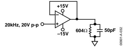
Figure 32. Output Swing,  $V_S = \pm 15\text{ V}$ ,  $G = +1$
