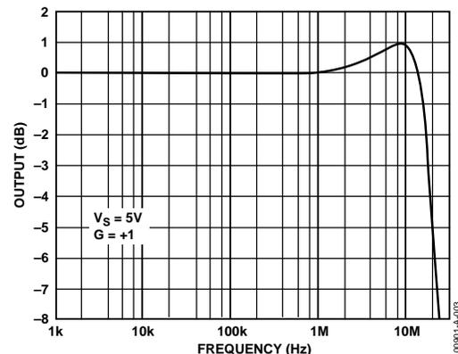
Figure 3. Small Signal Bandwidth,  $G = +1$
