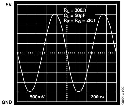
Figure 29. Output Swing,  $V_S = 5\text{ V}$ ,  $G = -1$
