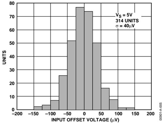
Figure 5. Typical Distribution of Input Offset Voltage
