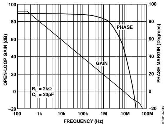
Figure 15. Open-Loop Gain and Phase vs. Frequency
