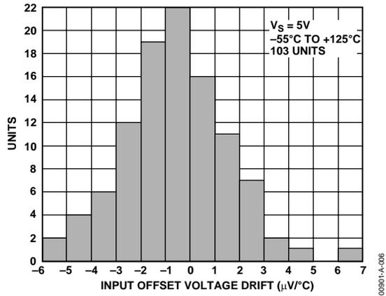
Figure 6. Typical Distribution of Input Offset Voltage Drift
