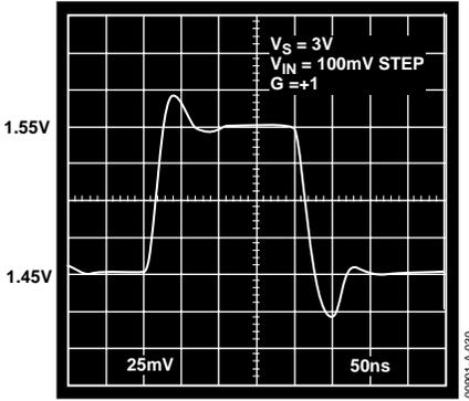
Figure 30. Pulse Response,  $V_S = 3\text{ V}$ ,  $G = +1$
