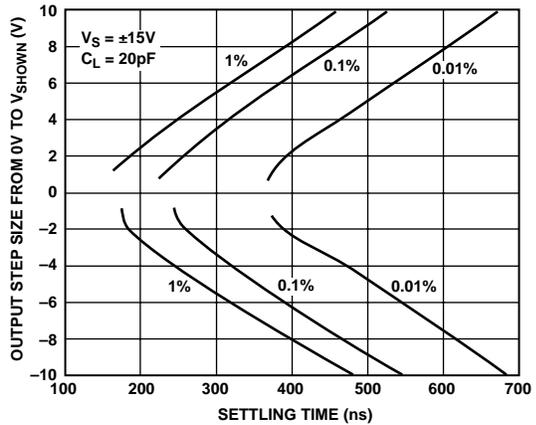
Figure 19. Inverter Settling Time vs. Output Step Size
