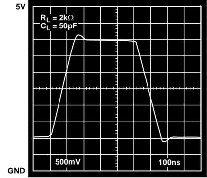
Figure 33. Pulse Response,  $V_S = 5\text{ V}$ ,  $G = +1$
