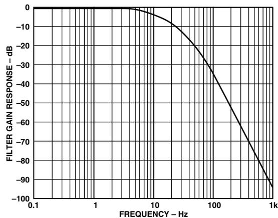
Figure 22. 10 Hz Sallen Key Low-Pass Filter
