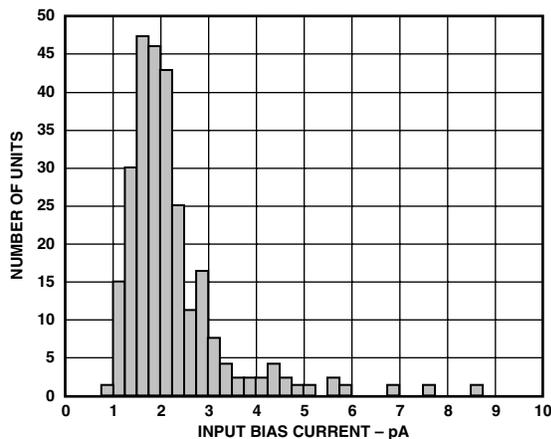
Figure 1. Typical Distribution of Input Bias Current
