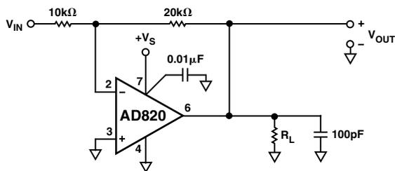
Figure 10. Gain of Two Inverter
