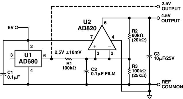
Figure 21. Single Supply 4.5 V Low Dropout Reference
