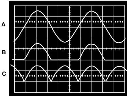
Figure 20. Single Supply Half- and Full-Wave Rectifier
