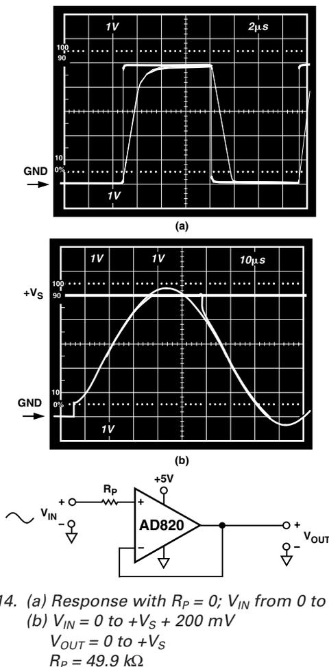
Figure 14. (a) Response with  $R_P = 0$ ;  $V_{IN}$  from 0 to  $+V_S$
