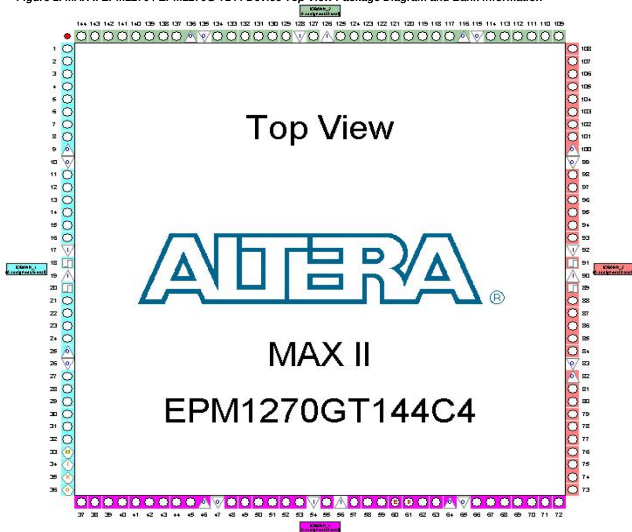
Figure 1. MAX II EPM1270 / EPM1270G T144 Device Top View Package Diagram and Bank Information
