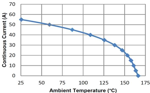
Figure 3: Maximum Continuous Current at a Given  $T_A$
