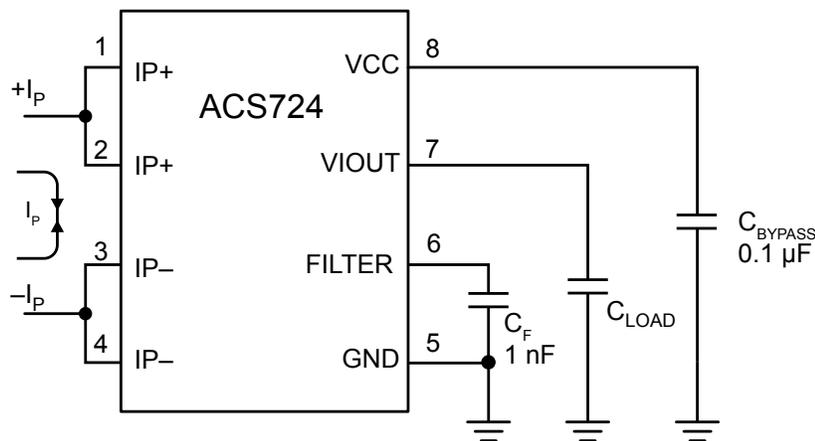
The ACS724 outputs an analog signal,  $V_{IOUT}$ , that changes proportionally with the bidirectional AC or DC primary sensed current,  $I_P$ , within the specified measurement range. The FILTER pin can be used to decrease the bandwidth in order to optimize the noise performance.
