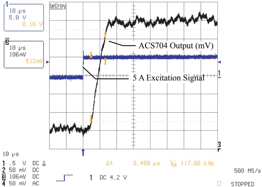
Typical Peak-to-Peak Noise of ACS704ELC-005 at  $T_A=25^\circ\text{C}$
