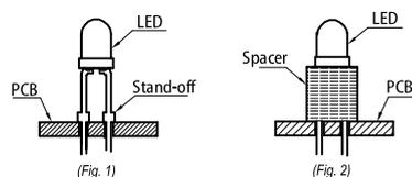
3. Use stand-offs (Fig. 1) or spacers (Fig. 2) to securely position the LED above the PCB.
