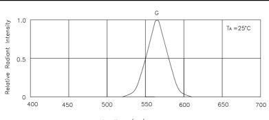
wavelength へ(nm) RELATIVE INTENSITY Vs. WAVELENGTH
