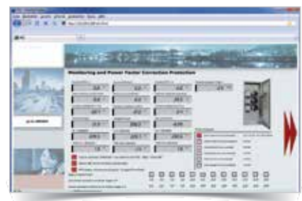
Fig.: Monitoring of limit values via UMG 604-PRO homepage
