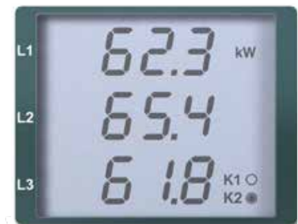
Fig.: Effective power, all three phases at a glance
