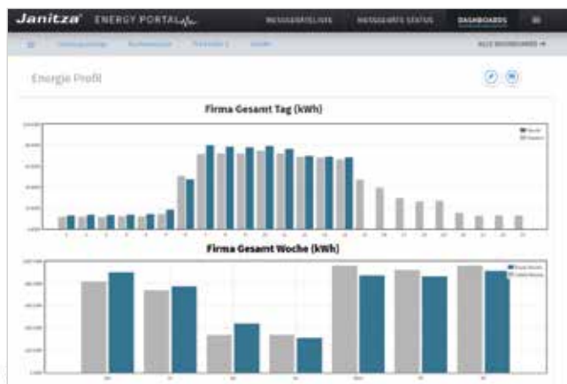
Fig.: Dashboard example with two bar charts to compare el. energy values from the current day with the previous day or the current week with the previous week.
