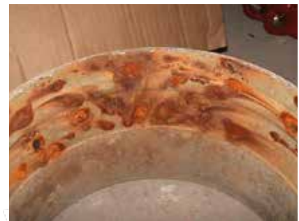
Fig.: Corrosion of pipes
