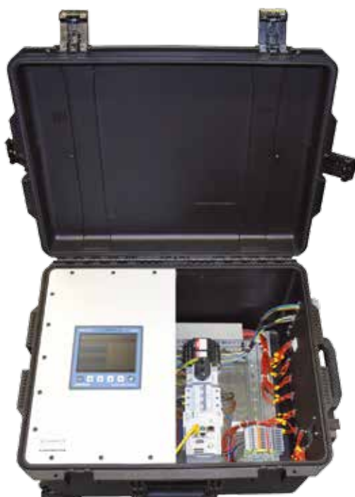
Fig.: Internal view of the mobile GridMonitor
