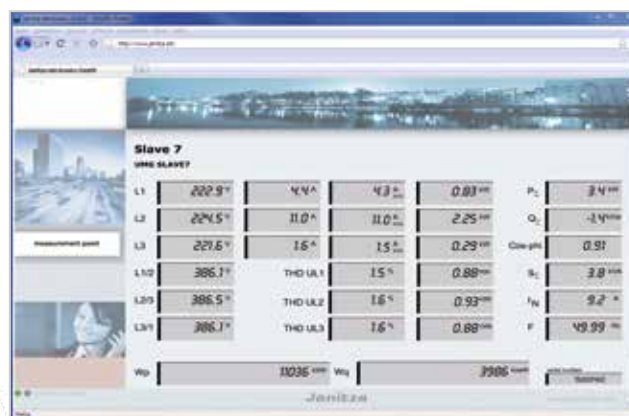
Fig.: Display of measured values for an individual slave device
