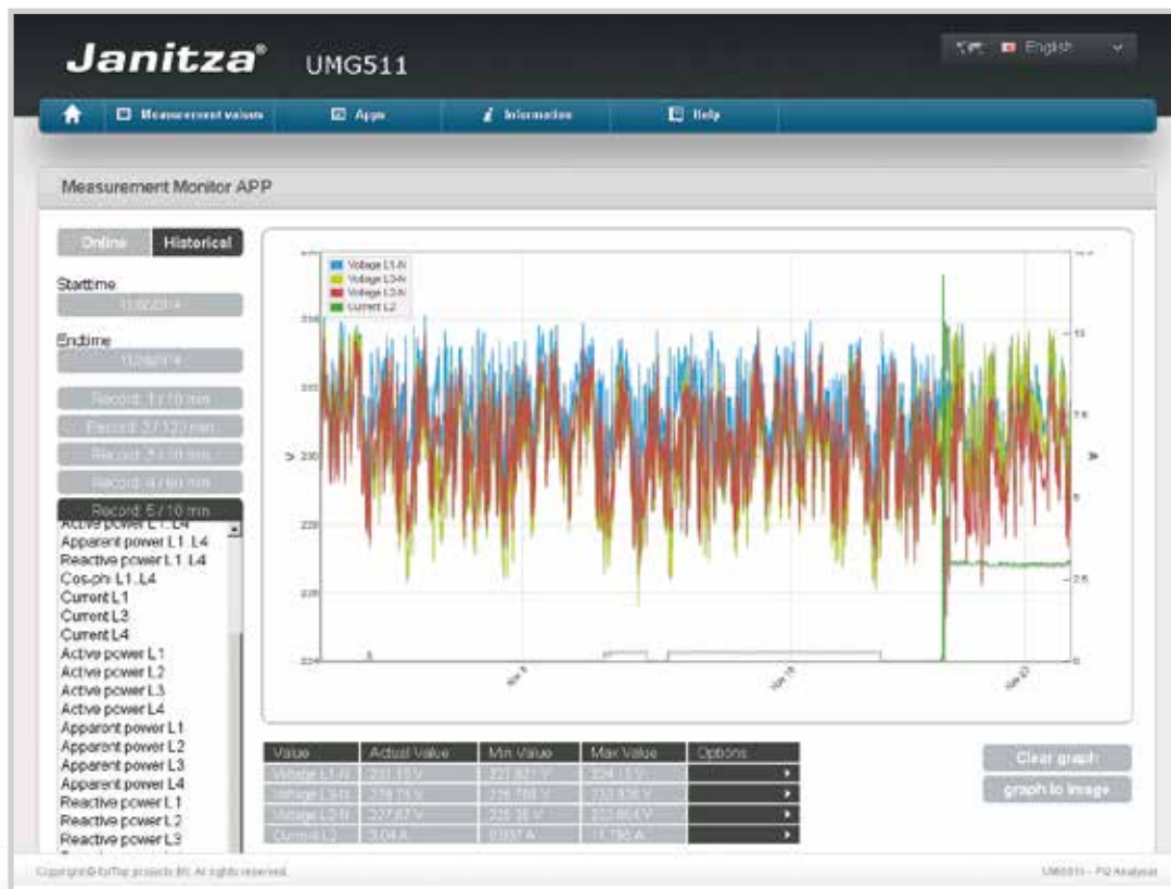
Fig.: APP Measurement monitor
