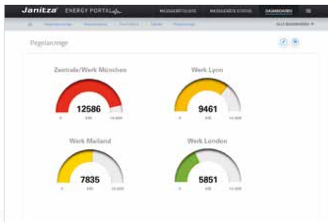
Fig.: Benchmark for the production sites with level displays. The limit values can be adjusted individually for each of the locations.
