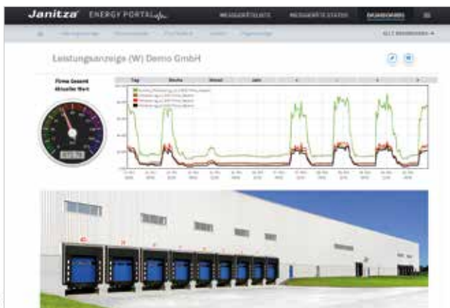
Fig.: Example of a dashboard with a line chart (load profile) and the power value displayed using an analogue pointer display.
