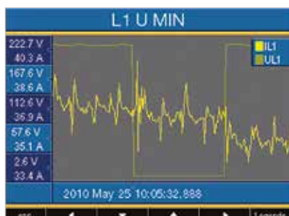
Fig.: Illustration of the full wave effective values for an event
