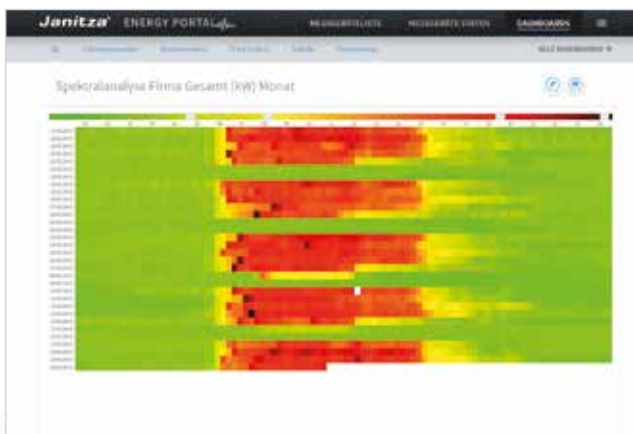
Fig.: Heat map (spectral analysis) to determine peak loads that drive costs. The scroll bar in the chart's header area can be used to adjust the threshold values individually.
