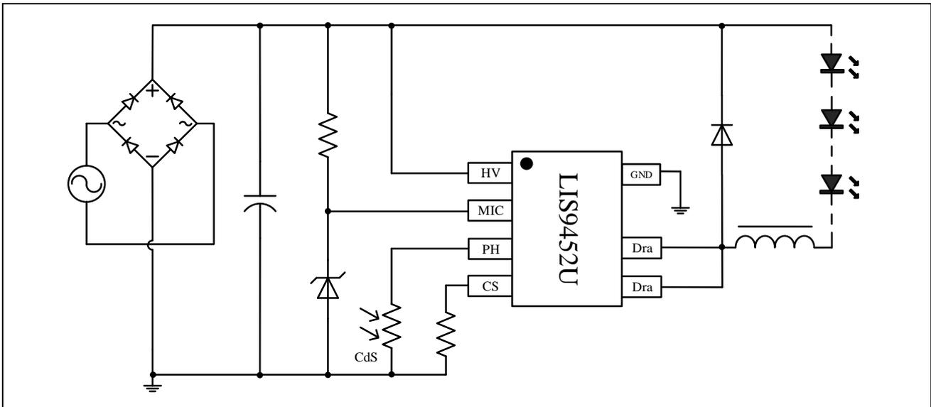
Figure2 Typical application diagram for the LIS9452U, sensitive to ambient luminous intensity only
