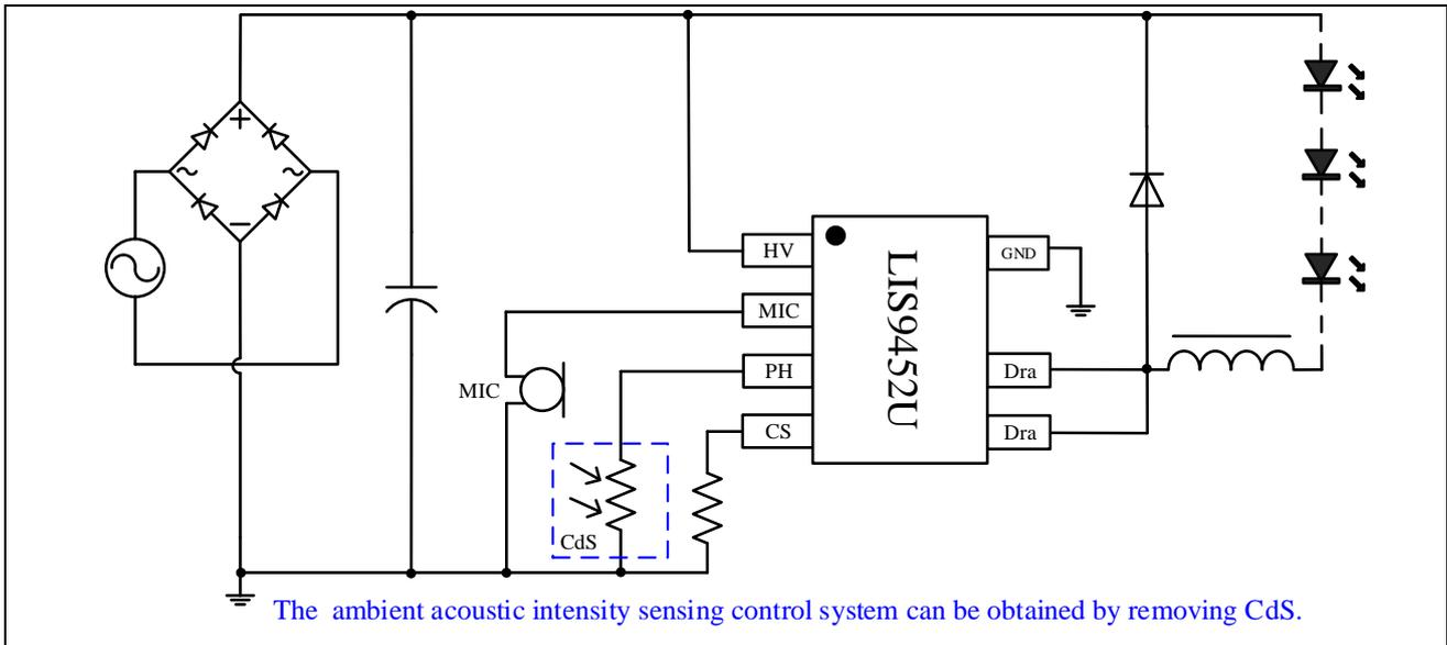
Figure1 Typical application diagram for the LIS9452U, sensitive to ambient acoustic and luminous intensity or to ambient acoustic intensity only (by removing the CdS photoresistor)
