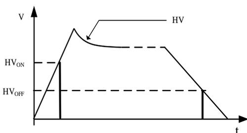
Figure 3 Hysteresis curve for the UVLO comparator
