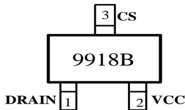
Figure 2. Pin configuration
