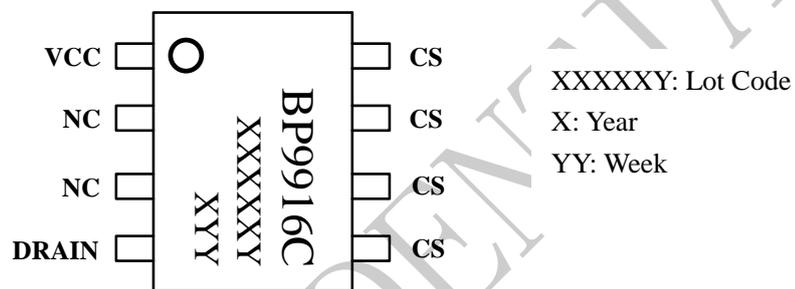
Figure 2. Pin configuration
