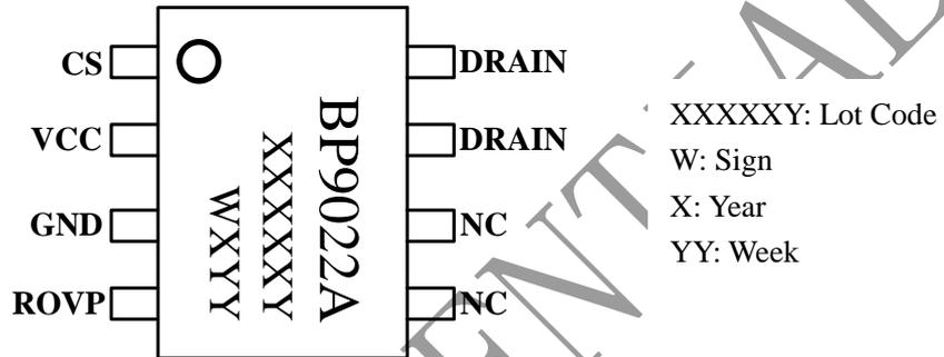
Figure 2. Pin configuration
