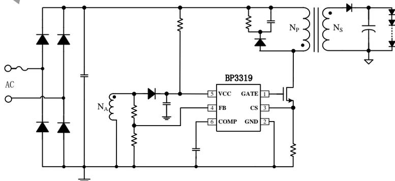
Figure 1. Typical application circuit for BP3319
