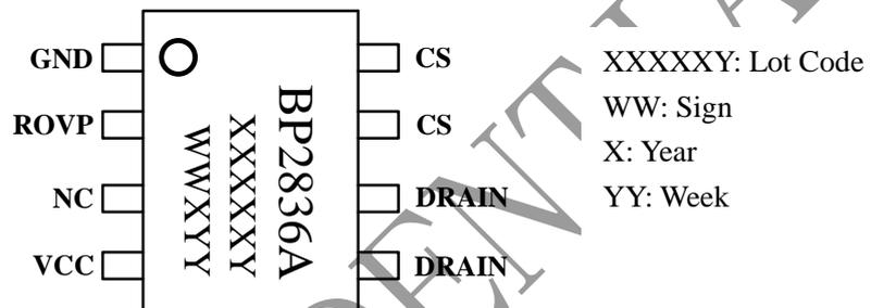
Figure 2. Pin configuration
