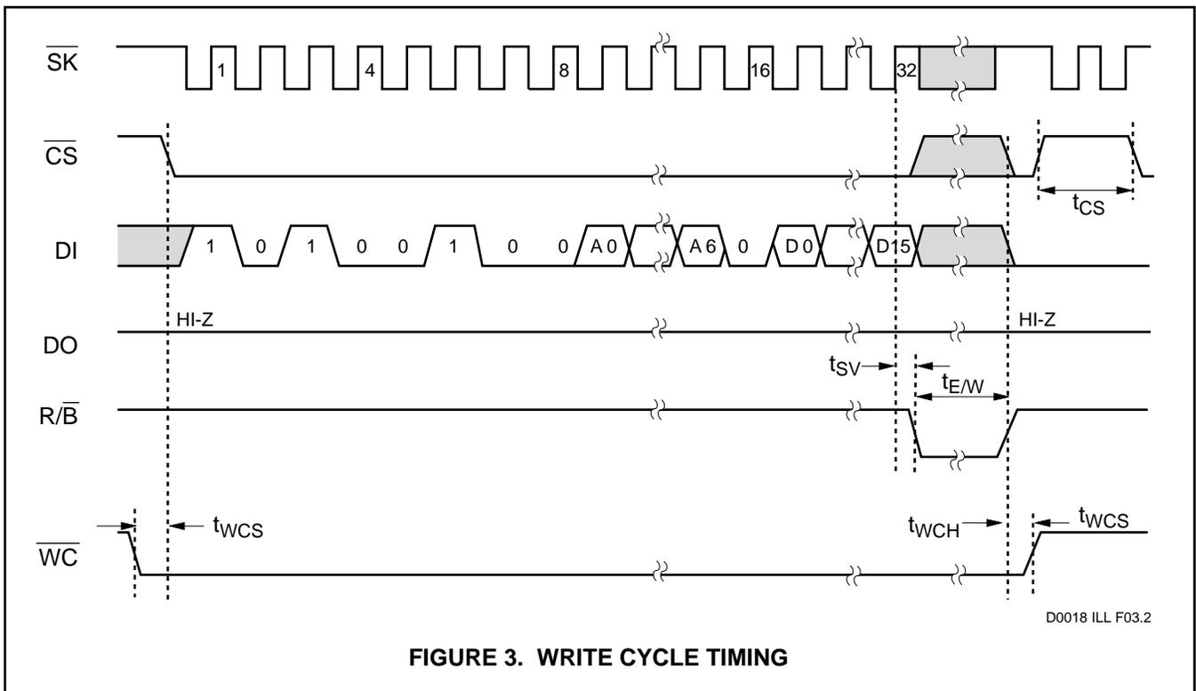
**FIGURE 3. WRITE CYCLE TIMING**
