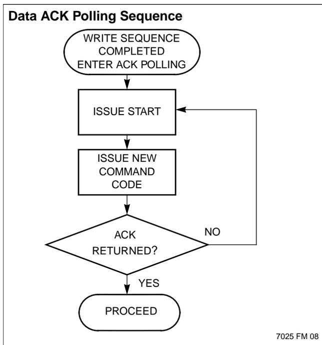
After the password sequence, there is always a nonvolatile write cycle. This is done to discourage random guesses of the password if the device is being tampered with. In order to continue the transaction, the X76F641
