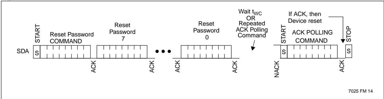
**Figure 10. Reset Device**
