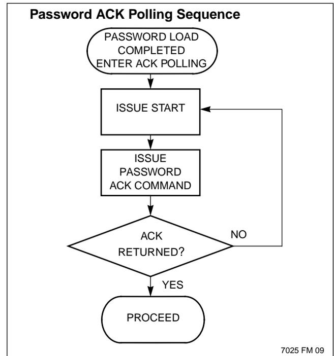
If the password that was inserted was correct, then an "ACK" will be returned once the nonvolatile cycle is over, in response to the ACK polling cycle immediately following it.
