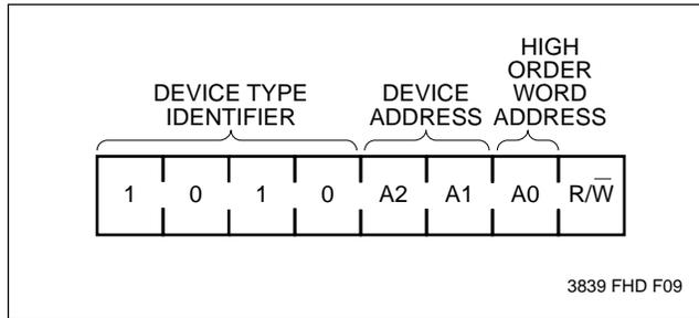
The next two significant bits address a particular device. A system could have up to four X24C04 devices on the bus (see Figure 10). The four addresses are defined by the state of the A<sub>1</sub> and A<sub>2</sub> inputs.
