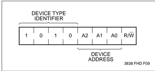
The next three significant bits address a particular device. A system could have up to eight X24C02 devices on the bus (see Figure 10). The eight addresses are defined by the state of the A<sub>0</sub>, A<sub>1</sub> and A<sub>2</sub> inputs.
