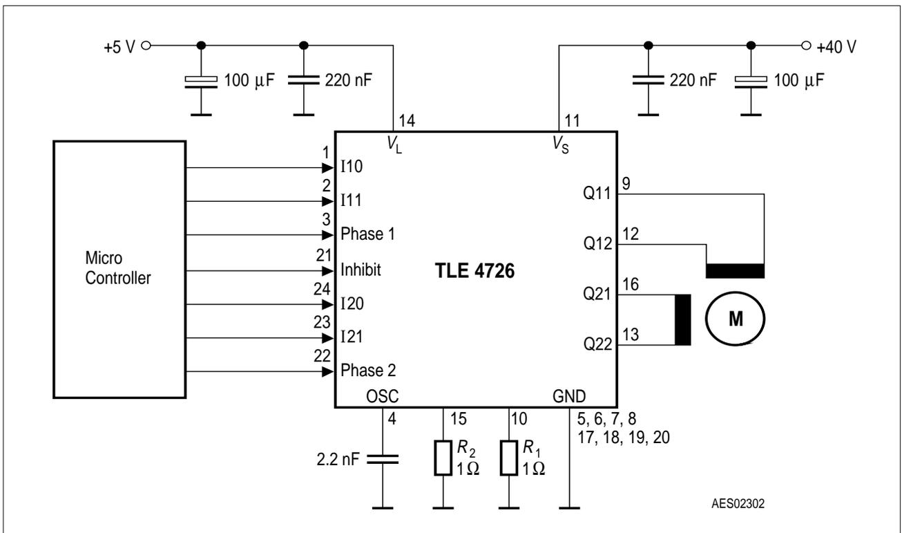
Figure 4 Application Circuit
