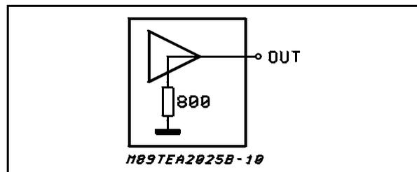
The TEA 2025B solution allows to save components because of such resistors (800 ohm) are included into the chip.
