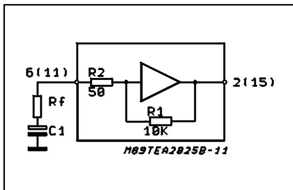
The bridge configuration is realized very easily thanks to an internal voltage divider which provides (at pin 1) the CH 1 output signal after reduction. It is enough to connect pin 6 (inverting input of CH 2) with a capacitor to pin 1 and to connect to ground the pin 7.
