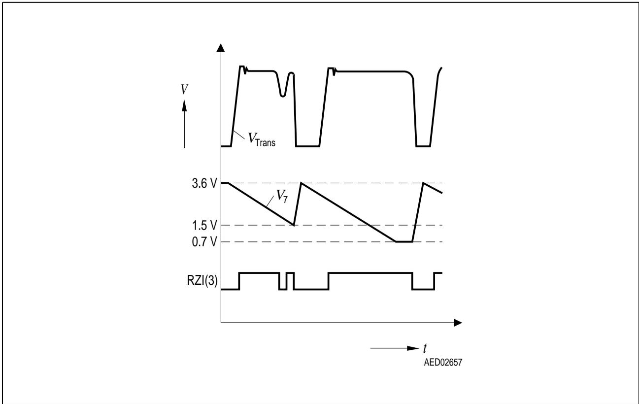
**Figure 12 Pulse Diagram for Fixed Frequency Circuit**
