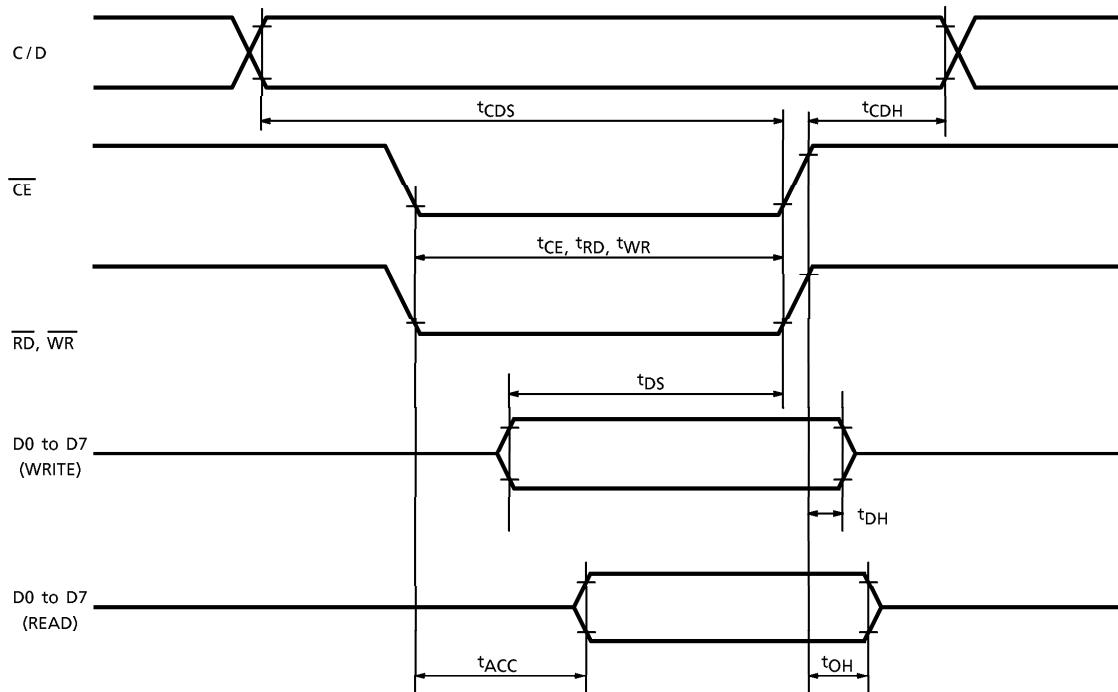
TEST CONDITIONS (Unless otherwise noted,  $V_{DD} = 5.0V \pm 10\%$ ,  $V_{SS} = 0V$ ,  $T_a = -20$  to  $75^\circ C$ )
