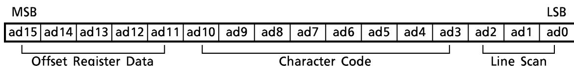
T6963C assign External character generator, when character code set 80H to FFH in using internal character generator. Character code 00H to 80H assign External character generator, when External generator mode.
