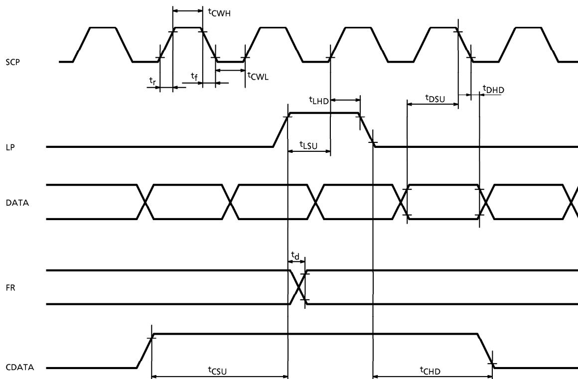
TEST CONDITIONS (Unless otherwise noted,  $V_{DD} = 5.0V \pm 10\%$ ,  $V_{SS} = 0V$ ,  $T_a = -20$  to  $70^\circ C$ )
