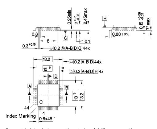
Does not include plastic or metal protrusion of 0.25 max. per side
