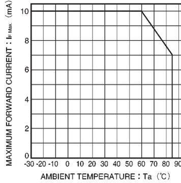
Fig. 6 Maximum forward current vs. ambient temperature
