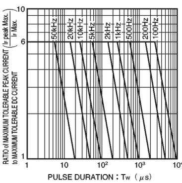
Fig. 5 Maximum tolerable peak current vs. pulse duration
