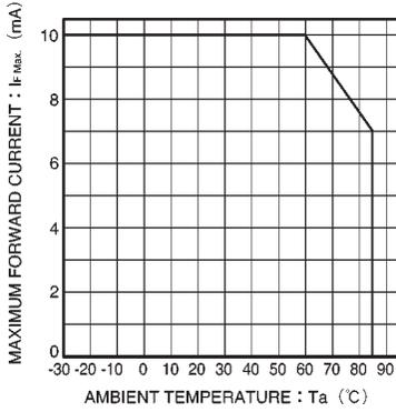
Fig. 6 Maximum forward current vs. ambient temperature
