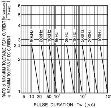
Fig. 23 Maximum tolerable peak current vs. pulse duration
