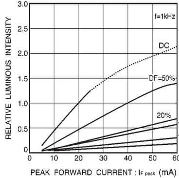
Fig. 24 Luminous intensity vs. peak forward current
