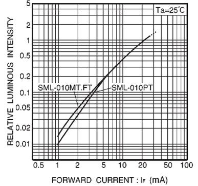
Fig. 28 Luminous intensity vs. forward current
