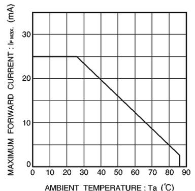
Fig. 31 Maximum forward current vs. ambient temperature
