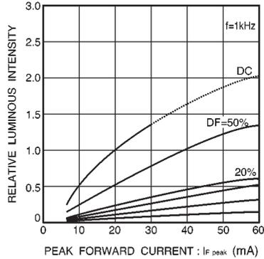
Fig. 6 Luminous intensity vs. peak forward current
