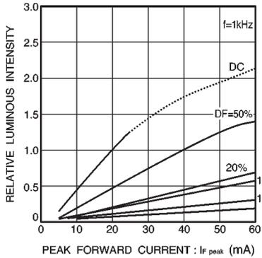
Fig. 12 Luminous intensity vs. peak forward current
