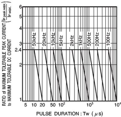
Fig. 11 Maximum tolerable peak current vs. pulse duration
