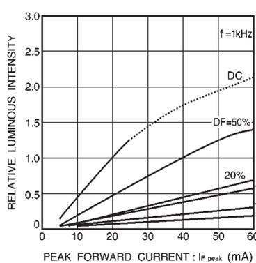
Fig. 18 Luminous intensity vs. peak forward current
