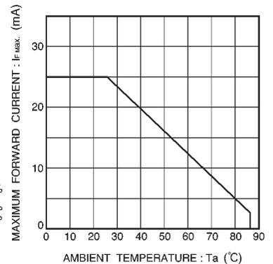
Fig. 19 Maximum forward current vs. ambient temperature
