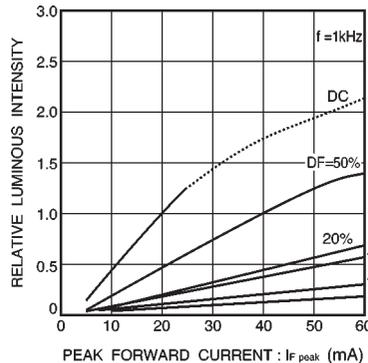
Fig. 30 Luminous intensity vs. peak forward current
