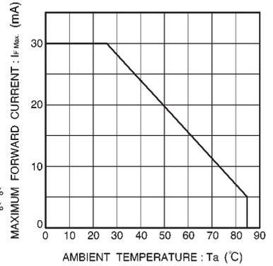
Fig. 7 Maximum forward current vs. ambient temperature
