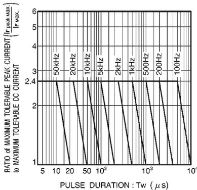
Fig. 29 Maximum tolerable peak current vs. pulse duration
