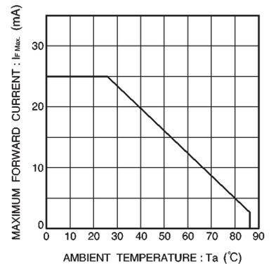
Fig. 13 Maximum forward current vs. ambient temperature
