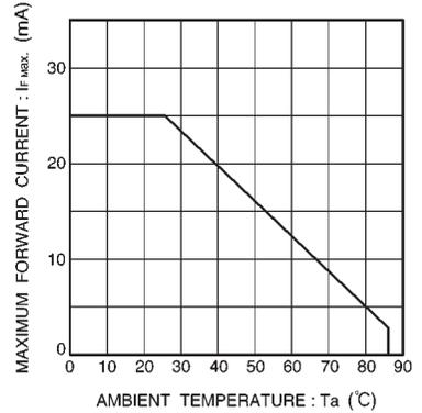
Fig. 25 Maximum forward current vs. ambient temperature
