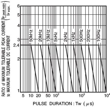
Fig. 17 Maximum tolerable peak current vs. pulse duration
