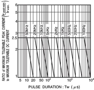
Fig. 5 Maximum tolerable peak current vs. pulse duration
