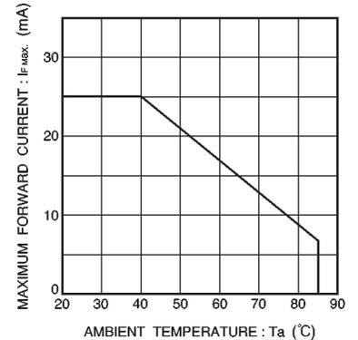
Fig. 26 Maximum forward current vs. ambient temperature
