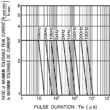
Fig. 6 Maximum tolerable peak current vs. pulse duration
