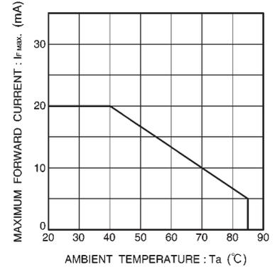
Fig. 14 Maximum forward current vs. ambient temperature
