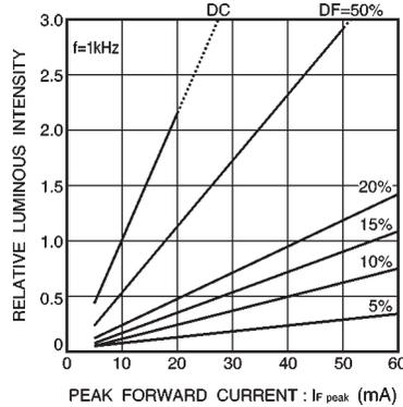
Fig. 19 Luminous intensity vs. peak forward current
