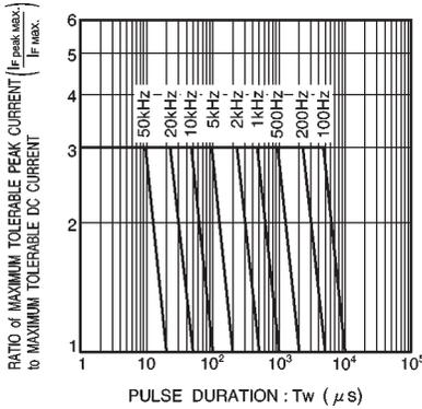
Fig. 18 Maximum tolerable peak current vs. pulse duration
