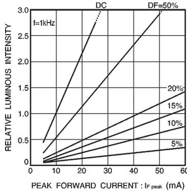
Fig. 25 Luminous intensity vs. peak forward current
