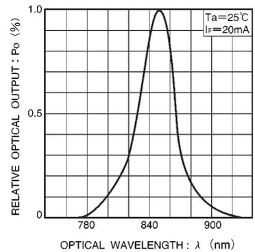
Fig. 3 Wavelength characteristics
