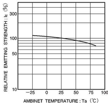
Fig. 5 Relative emitting strength vs. ambient temperature
