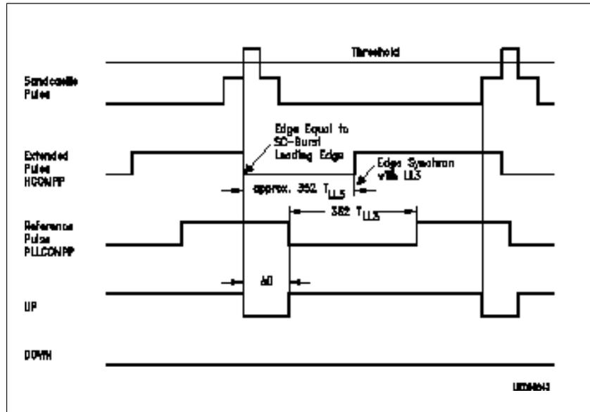
Function of SC-Pulse Extension and Phase Comparison
