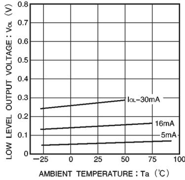
Fig.5 Low level output voltage vs. ambient temperature
