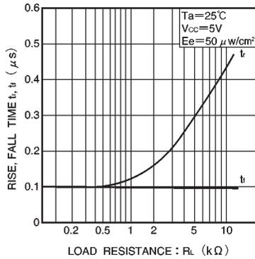
Fig.7 Rise and fall time vs. load resistance
