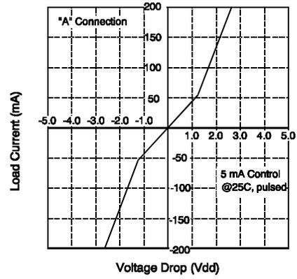
Figure 2. Linearity Characteristics
