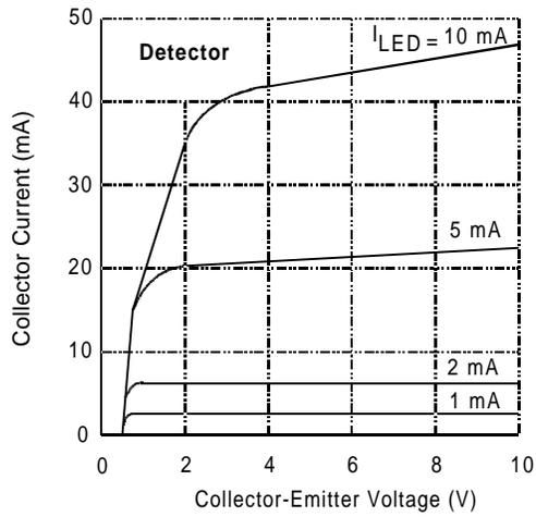
Figure 9. Typical Transfer Characteristics
