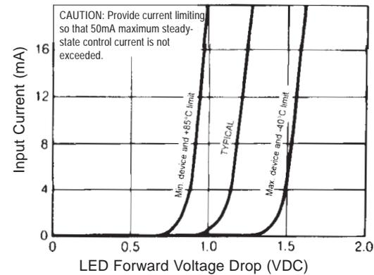
Figure 5. Input Characteristics
