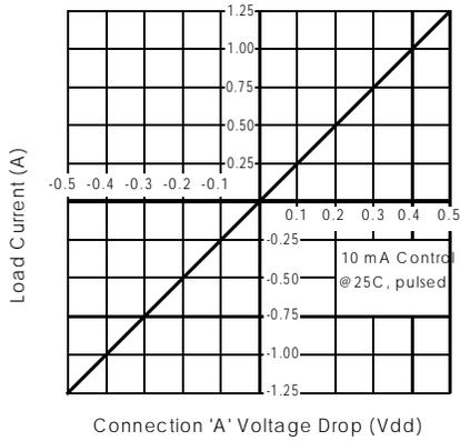
Figure 3. Linearity Characteristics
