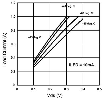
Figure 3. Typical On-Characteristics
