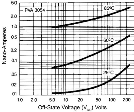
Figure 5. Typical Variation of Off-State Leakage Current
