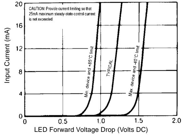
Figure 6. Input Characteristics
