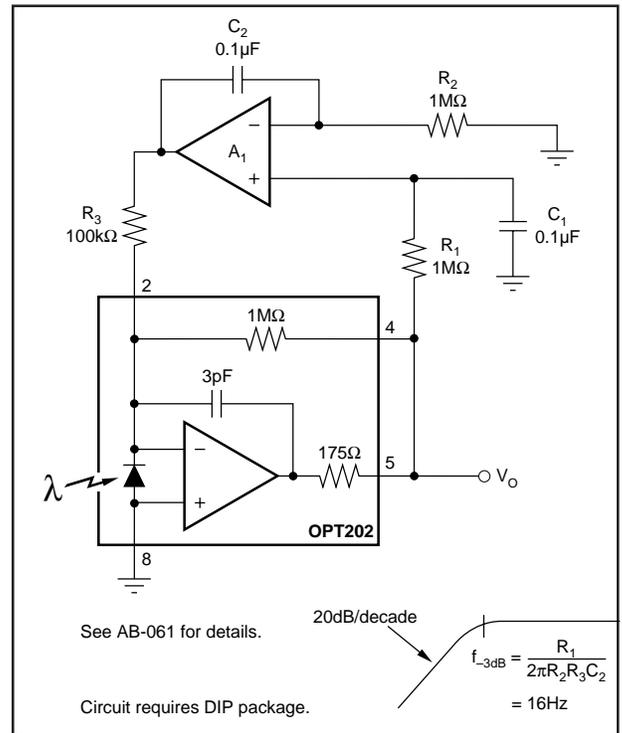
FIGURE 8. DC Restoration Rejects Unwanted Steady-State Background Light.
