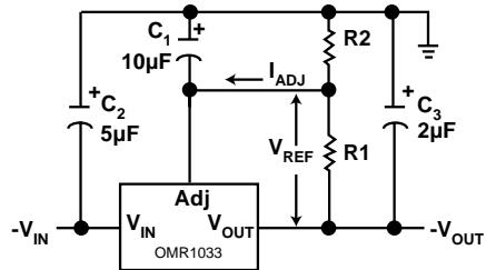
$$V_{OUT} = V_{REF} \left( 1 + \frac{R2}{R1} \right) + I_{ADJ} (R2)$$
