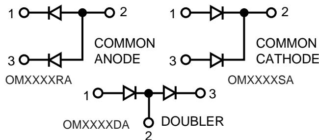
Common cathode is standard. Contact factory for performance characteristics for common anode and doubler.
