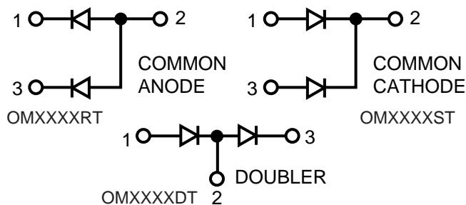
Common cathode is standard. Contact factory for performance characteristics
