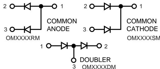
Common cathode is standard. Contact factory for performance characteristics for common anode and doubler.
