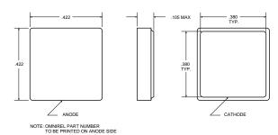
Maximum Soldering Temp = 250°C, 3 sec.
