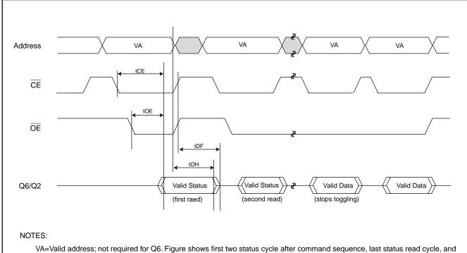
VA=Valid address; not required for Q6. Figure shows first two status cycle after command sequence, last status read cycle, and array data read cycle.
