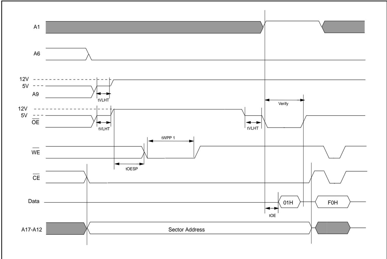
**TIMING WAVEFORM FOR CHIP UNPROTECTION FOR SYSTEM WITH 12V**
