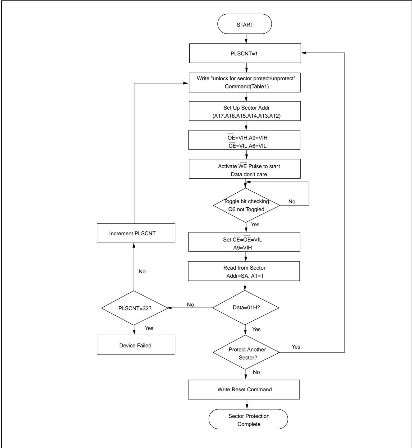
**CHIP UNPROTECTION ALGORITHM FOR SYSTEM WITHOUT 12V**
