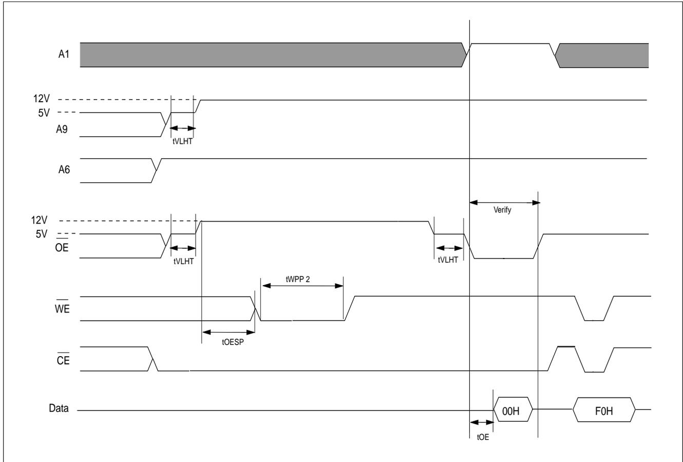
**SECTOR PROTECTION ALGORITHM FOR SYSTEM WITH 12V**
