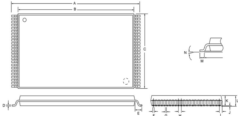
**NOTE:** Each lead centerline is located within .25 mm [.01 inch] of its true position [TP] at maximum material condition.
