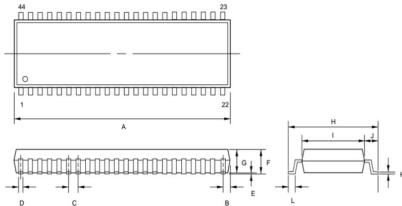
**NOTE:** Each lead centerline is located within .25 mm [.01 inch] of its true position [TP] at maximum material condition.
