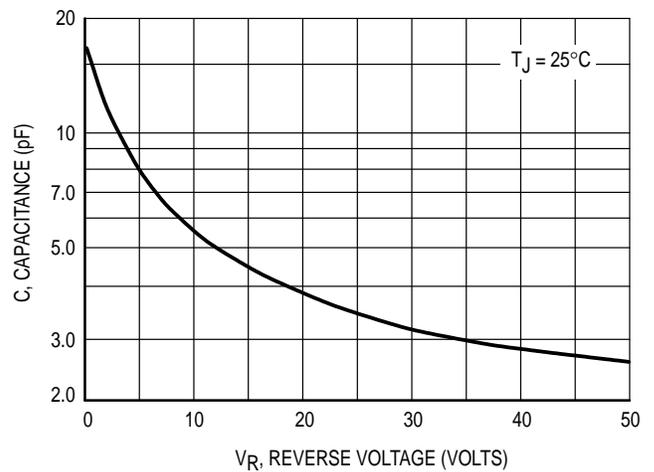
Figure 5. Typical Capacitance
