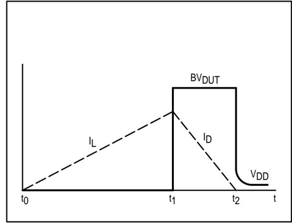
Figure 7. Current–Voltage Waveforms
