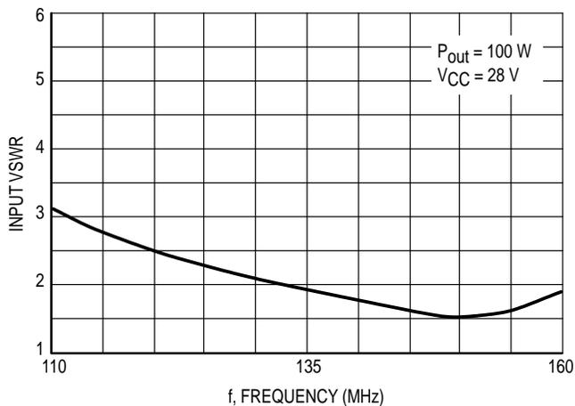
**Figure 4. Input VSWR versus Frequency
