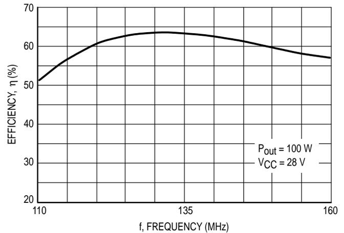
**Figure 3. Efficiency versus Frequency
