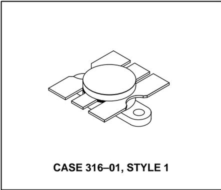
The MRF247 is designed for 12.5 Volt VHF large-signal amplifier applications in industrial and commercial FM equipment operating to 175 MHz.
