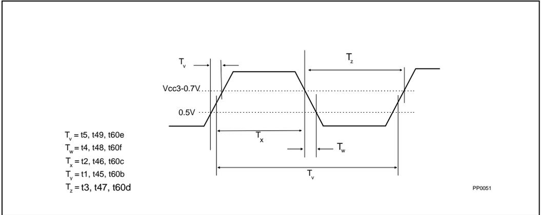
Figure 3. Clock Waveform
