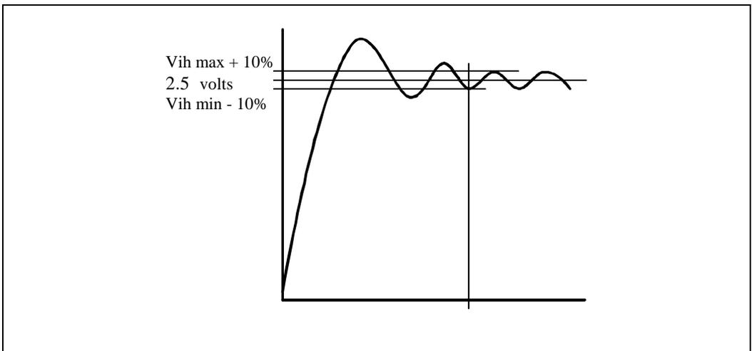
Figure 13. Settling Time
