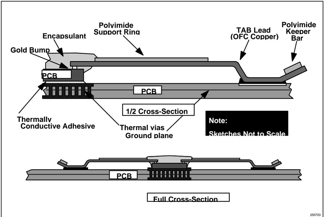
Figure 18. Cross-Sectional View of the Mounted TCP
