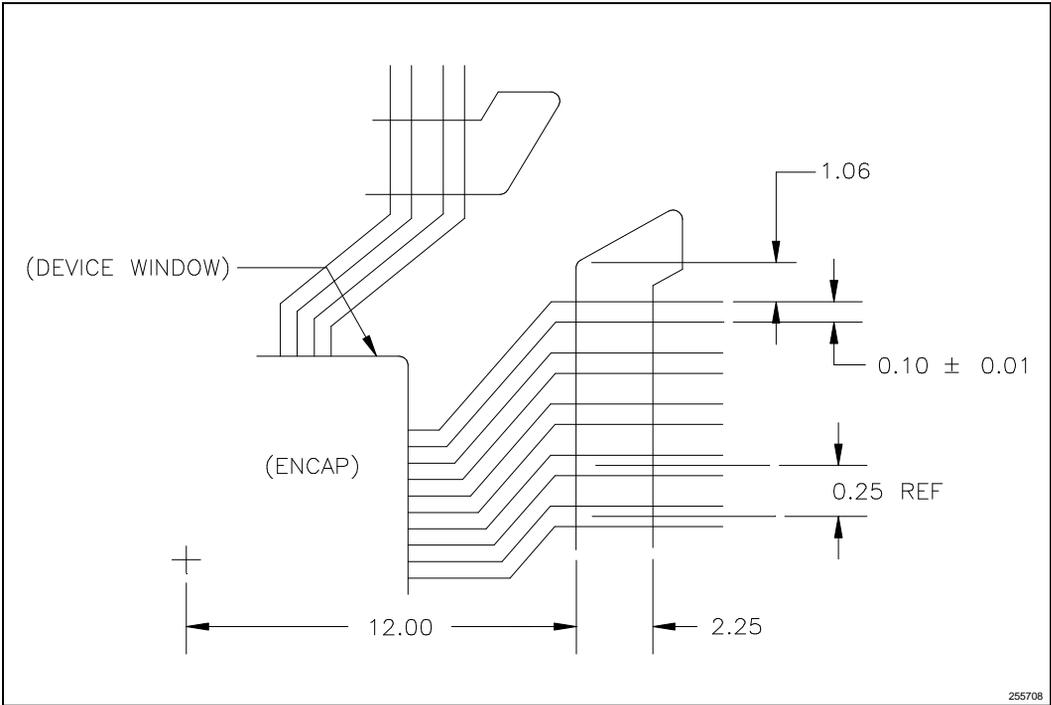
Figure 22. Outer Lead Bond (OLB) Window Detail
