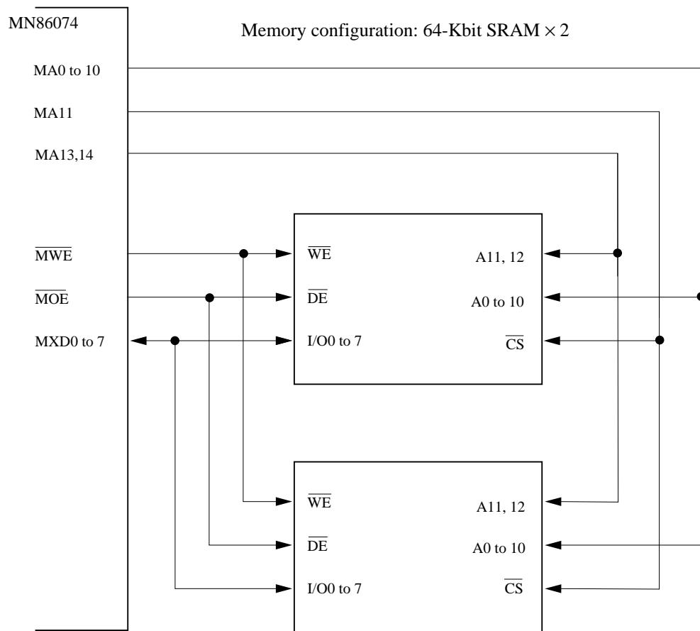
**■ Application Circuit Example #3: Line lengths of 4097 to 8192 pixels**
